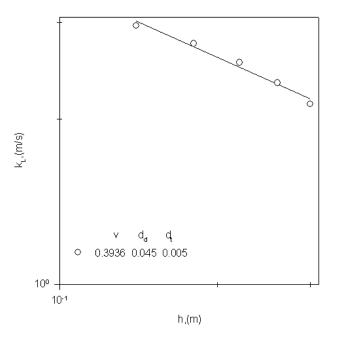
Figure 12: Variation of mass transfer coefficient with distance of disc
