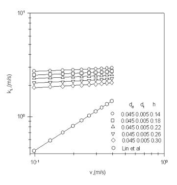
Figure 11: Variation of mass transfer coefficient with velocity of electrolyte
