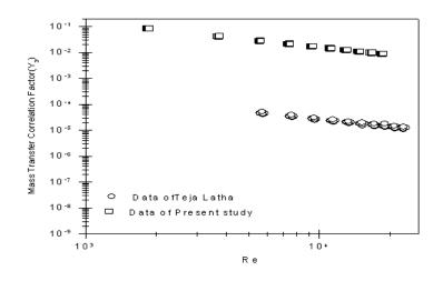
Figure 15: Variation of CFR with Re -Comparison plot
