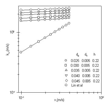
Figure 5: Variation of mass transfer coefficient with velocity - Effect of diameter of perforated disc
